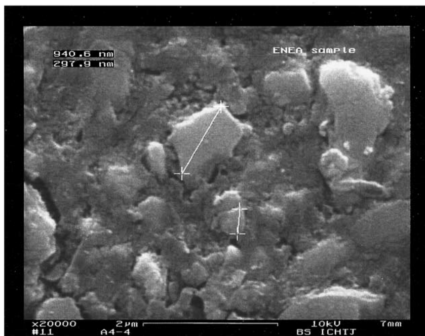
Figure 11 SEM photomicrographs of polished cross section of sol-gel and ENEA samples \text{Li}_2\text{TiO}_3 (see Fig. 10) used for tritium release rate measurements from different \text{Li}_2\text{TiO}_3 samples.
